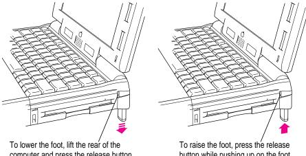
computer and press the release button. The foot extends automatically.
